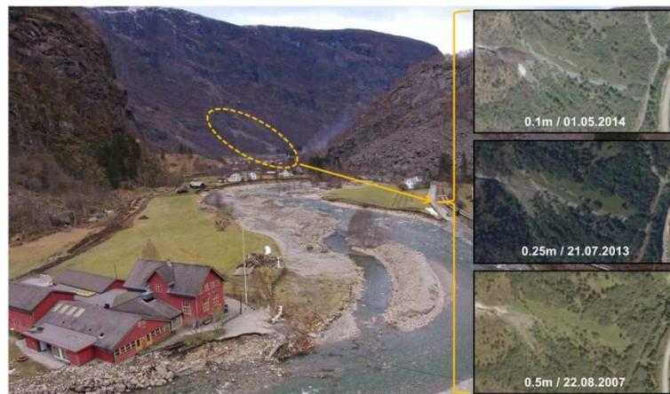
Figure 2: Photo (© Pål Ringkjøb Nielsen) from the Flåm valley and orthophotos from 2007, 2013 and 2014 showing changes in debris accumulation area.
